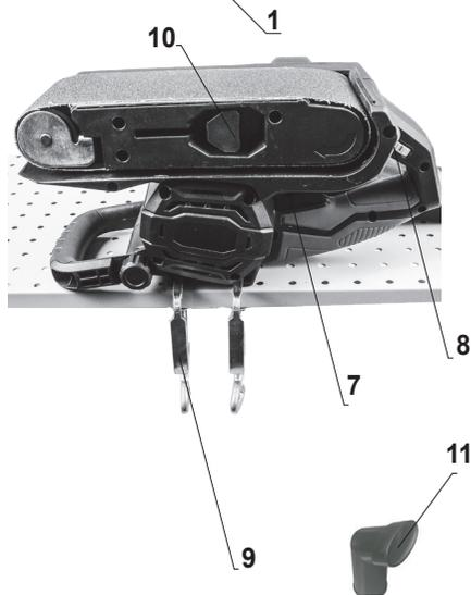
1. Swivel to adjust the position of the sandpaper sanding belt.
