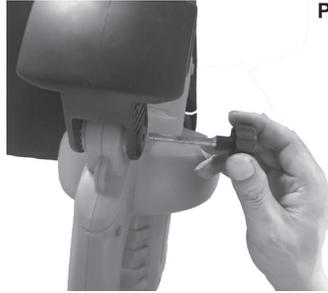
Fitting the adjustable handle (Pic.4)
