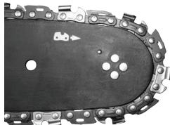
Move the guide bar away from the driving chain wheel, so chain guiding links are placed in the guide bar groove.
